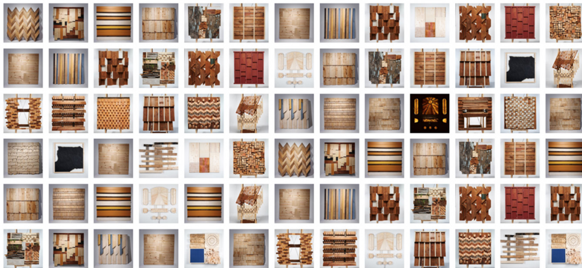
Fig 16] Examples of façade panels made out of reclaimed wood: Nordic Waste Wood for Good project.
