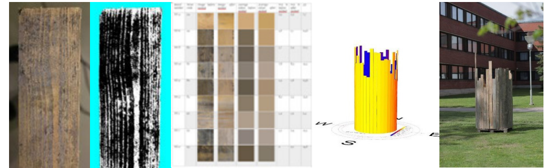
Fig 14 Architectural design from upcycled formwork wood, from physical object via computer vision techniques to simulation and real-world application.
