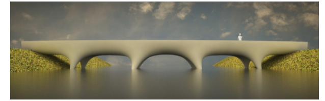
Fig[07] Concrete 3D printed bridge design.
