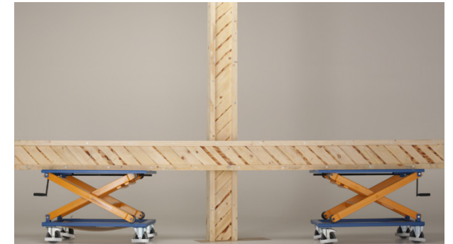
Fig 11 | Brusenius assembly – post and beam.
