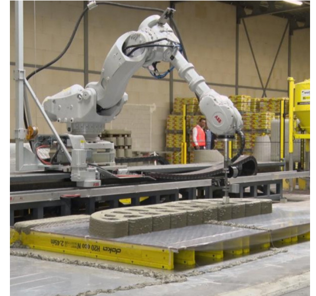
Fig[08] 3D printing of concrete using robotic production methods.
